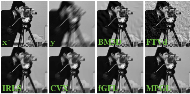
Figure 2: Visual quality comparison of image deconvolution on Cameraman. A local part is enlarged for visualization. Our result has a clearer background and sharper details than the others.
