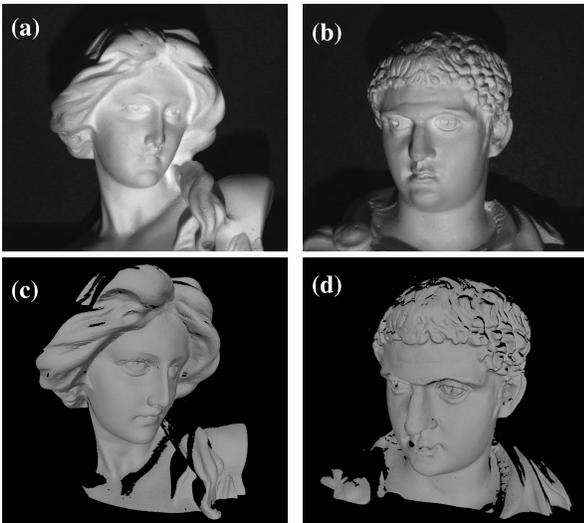
Fig. 10. More experimental results on real-world complex surfaces. (a) and (b) Photograph of the measured sculptures. (c) and (d) Reconstructed surfaces.
